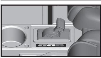
**IMPORTANT!** To avoid damaging the motors and gears, stop the vehicle before shifting from forward  $\clubsuit$  to reverse B.
